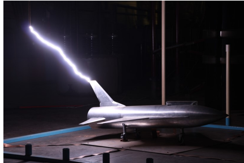
Aircraft model subject to “lightning like” situation
