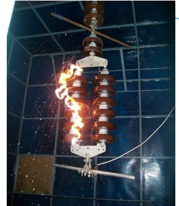
Insulator strings in transmission lines: pollution effects
